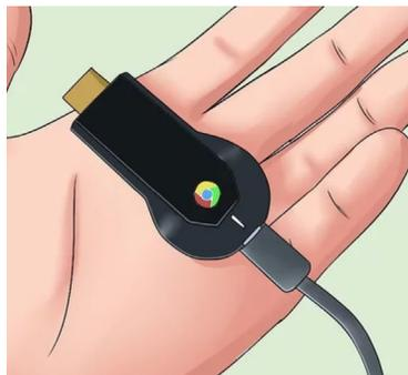
**Insert the USB port into the back of the Chromecast.** If you are using the USB port to charge the device, connect the USB cable to the device. If not, plug the device charger into it instead.
