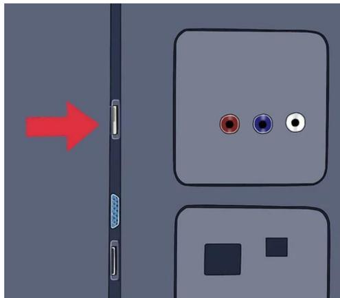
**Identify the HDMI port in the back or side of your HD TV.** You should also find whether or not your TV has a USB port for charging the device. If not, it will need an outlet or power strip nearby.
