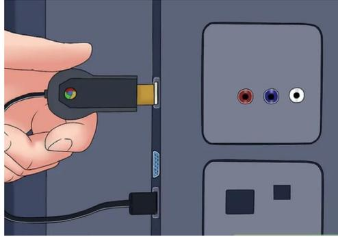
**Insert the other end of the Chromecast into the HDMI port.** The Chromecast connects directly to an HDMI port on your TV and stays hidden behind your TV or off to the side.
